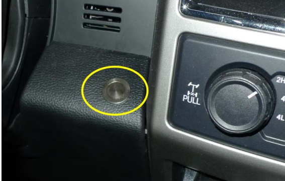
Figure 16: Horn Button Installed in Dash
